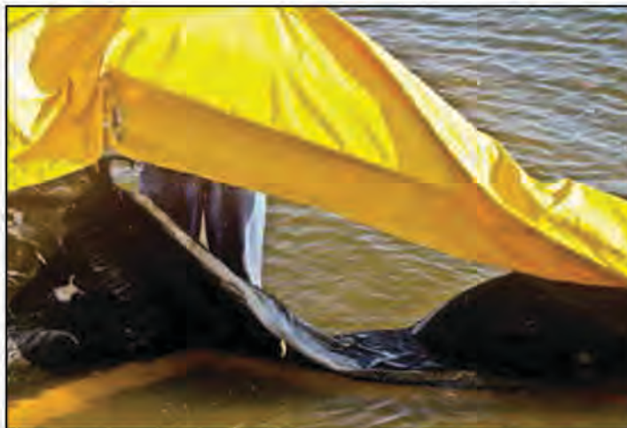
Tear between the float and the skirt. Image courtesy of GEI Works.
