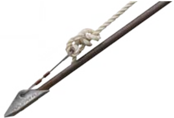
Step 6: Keeping the rope taut, thrust the driving rod sharply into the ground.
