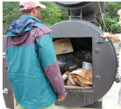
**System Capacity:** 4.2 MMBtu/hr waste combustion, providing 363-605 lb/hr (95165-275 kg/hr) processing capacity for mixed waste streams with an average gross HHV of up to 5500-8500 Btu/lb.
